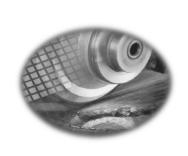
Die are saw cut from the wafer, assembled onto substrates where final package configuration is completed
